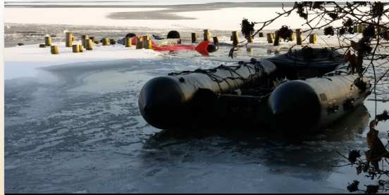
Vehicle recovery using underwater lift bags
